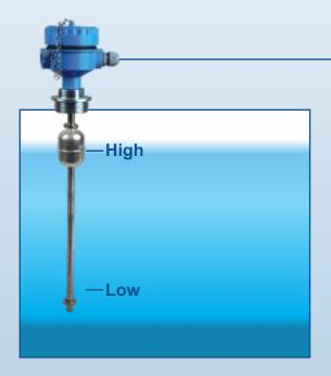
The controller has provision to select pump mode as Pump UP or Pump Down In Pump UP mode, the pump starts at Low Level & Stops at High Level. Pump UP mode is used to Fill the tank.
